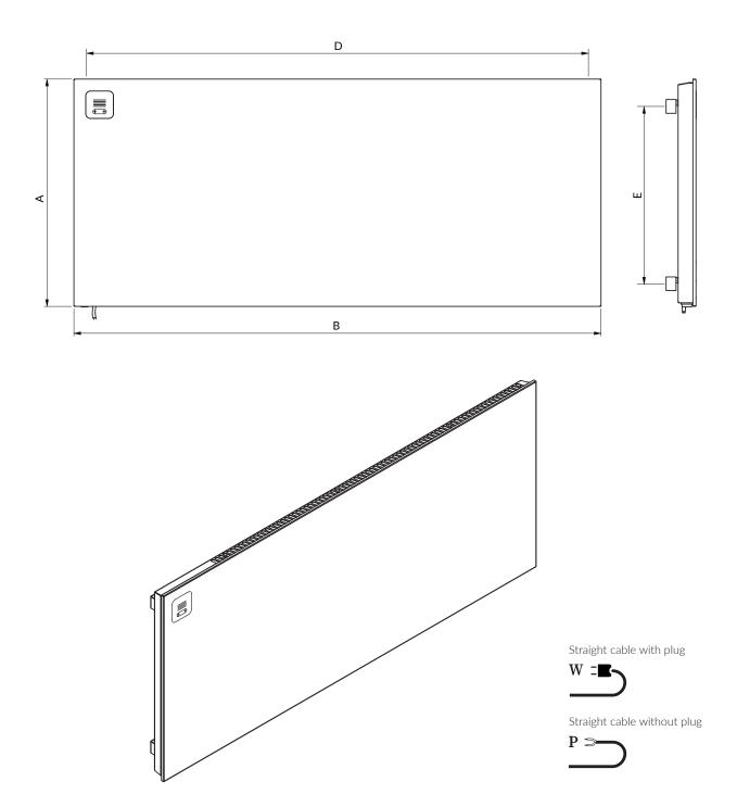
${\sf A-Height\ B-Width\ D-Horizontal\ distance\ between\ mounting\ bracket\ centres\ \ E-Vertical\ distance\ between\ mounting\ brackets}$
